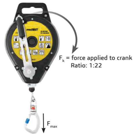
At load weight ( F_{max} ) of 140 kg force applied to the crank ( F_k ) shall be 6.3 kG.
